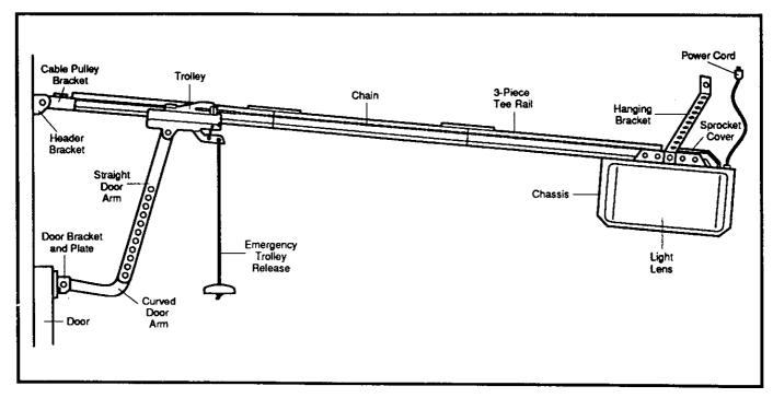
IT IS RECOMMENDED THAT THE OPENER BE INSTALLED 7 FEET OR MORE ABOVE FLOOR WHERE SPACE PERMITS. CERTAIN INSTALLATION PROCEDURES VARY ACCORDING TO GARAGE DOOR TYPES. WHERE THE DIFFERENCES OCCUR, BE SURE TO FOLLOW ONLY THOSE INSTRUCTIONS WHICH APPLY TO YOUR DOOR CONSTRUCTION.
